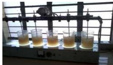
Figure 4 Schematic view of Conventional Jar Test Apparatus
